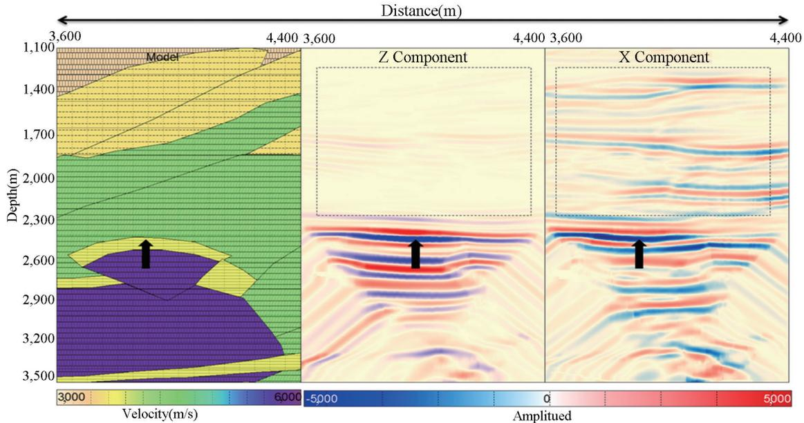
**Figure 8** Display Shows the Model on Left, Depth Migrated P-Wave in the Middle and Depth Migrated P-S Seismic Sections on the Rightmost Panel. Shallow Reflectors Are Better Imaged in P-S Seismic Section
