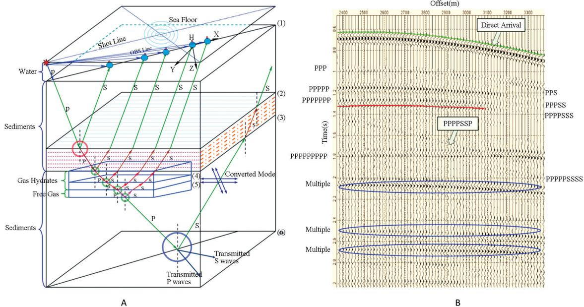
**Figure 9** Marine Environment Model and Generated Synthetic Seismogram With Identified P-S Wave Reflections. (A) The Model Consists of Water, Sedimentary Layer Target Layers Consist of Gas Hydrates and Free Gas. (B) Display of Identified P-S Wave Reflections That With Correlation of the Model. PPP Refers to Down-Going PP-Wave and Reflected P-Wave. PPS Refers to Down-Going PP and Reflected S-Wave
